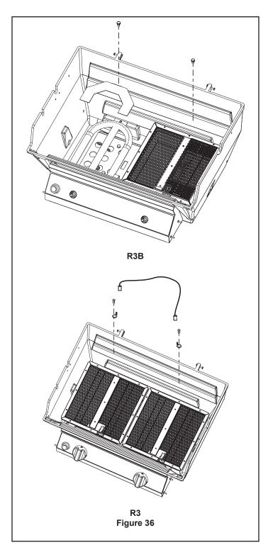
Remove LP burner orifices marked 1.25 mm for R3B. Remove LP burner orifice marked 1.3 mm for R3. See Figure 37.
